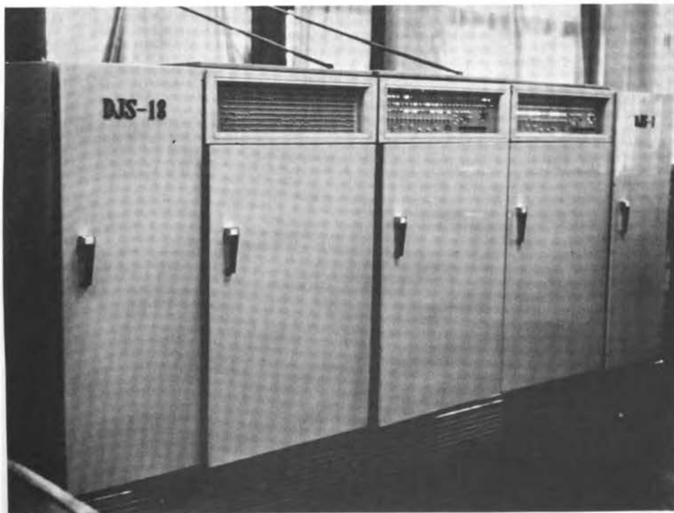
The central processing unit of the DJS-18 computer, constructed and installed in the Computer Center of Beijing University.
