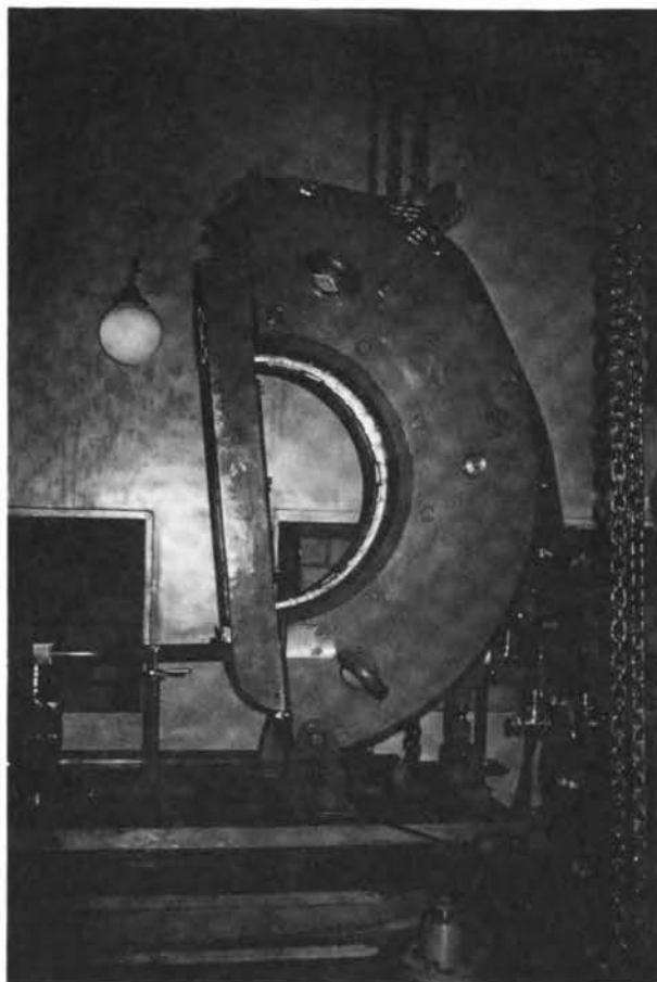
A large n = \frac{1}{2} spectrometer magnet constructed for use with the IMP cyclotron.
