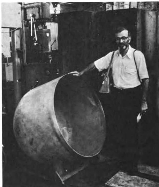
Alex Zucker examines an aluminum pressing that will subsequently form the dome for either a 2.5-MV Van de Graaf or a 3-MV Dynamitron produced in the Vanguard factory. The press used in producing these domes is shown at the left.
