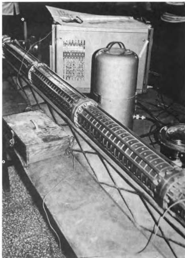
The prototype electron linear accelerator developed at Qinghua University with support from the Beijing Municipality. The stacked electrodes are here contained within a glass vacuum system.
