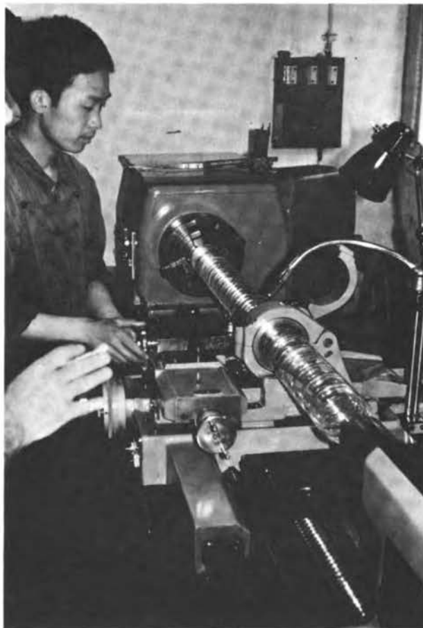
A young machinist in the Vanguard factory uses a high-quality Chinese-made lathe to produce lucite-insulating members. The delegation was surprised to find that the corrugations in these members were being developed freehand by the machinist.
