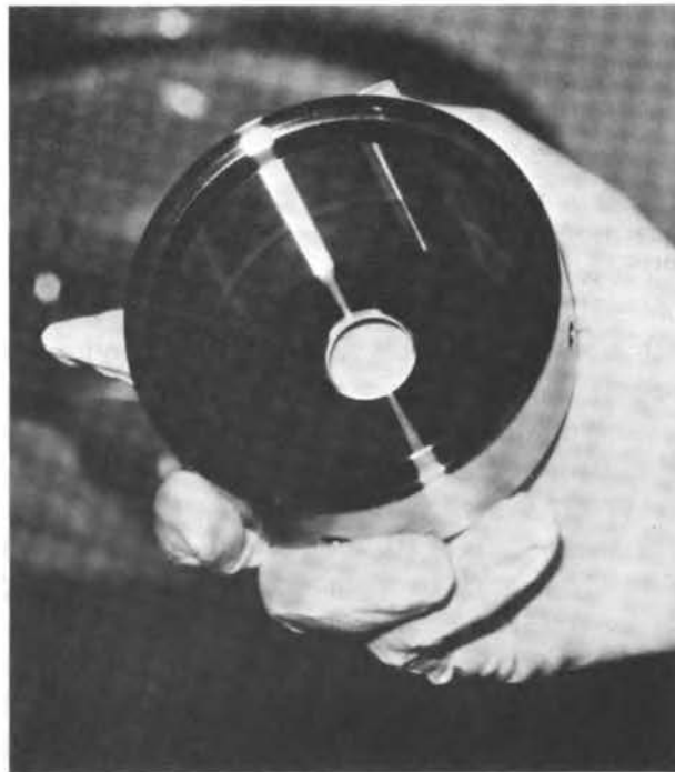
A completed linac diaphragm unit, produced as in the preceding illustration. The quality of the workmanship is outstanding—so much so that these units require no further grinding or polishing as they come from the production lathes.
