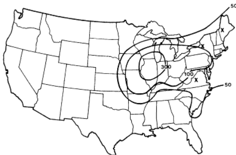
Figure 5.10 Average zinc deposition by precipitation over the continental United States, September 1966 to March 1967 (in grams per hectare per month). Source: Galloway et al. (1981); data from Lazrus et al. (1970).
