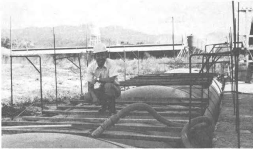
FIGURE 4.6 A biogas generator fabricated from reinforced plastic. The wood and metal racks can be weighted to increase gas pressure. (Lupton Engineering Corp.)
