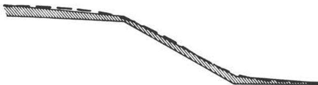
FIGURE 1.4 Schematic illustration of a kinematic cascade used for computing overland flow from a convex-concave hillslope. The hillslope indicated by the dashed line, and its approximation as a series of planes, is represented by the lower solid line. The shaded area shows the sheet of overland flow.
