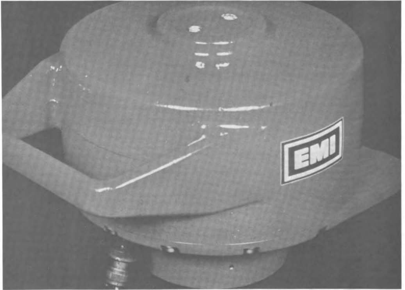
Figure 7 Laser-based system for wave-height measurement
