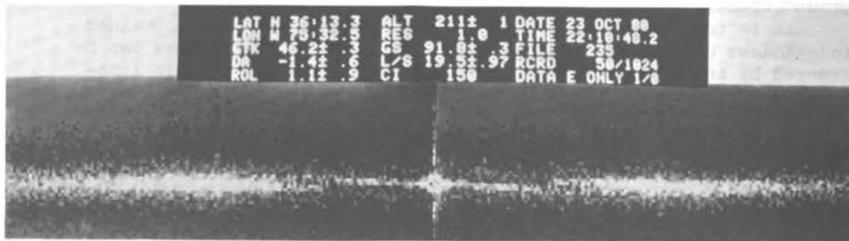
Figure 7 Grey-scale-coded variance spectrum before corrections for geometric distortion and rotation (to orient with respect to true north)
