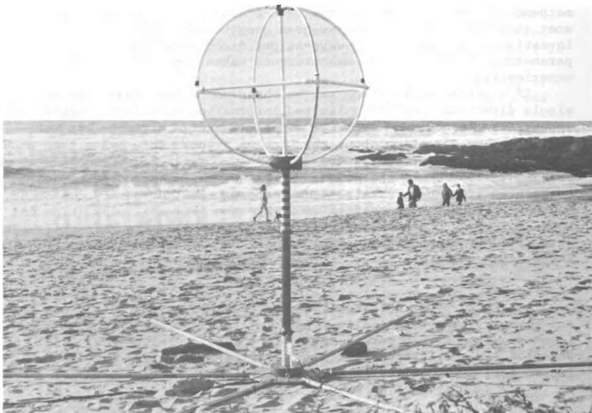
Figure 2 Photograph of compact crossed-loop/monopole antenna system for coastal wave-height directional spectral measurements, as operated at Pescadero, California, during January 1978. The antenna is less than 2 m tall.
