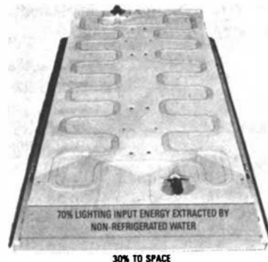
FIGURE 6 Lighting fixture incorporates nonrefrigerated water uniformly circulate to carry off heat.
