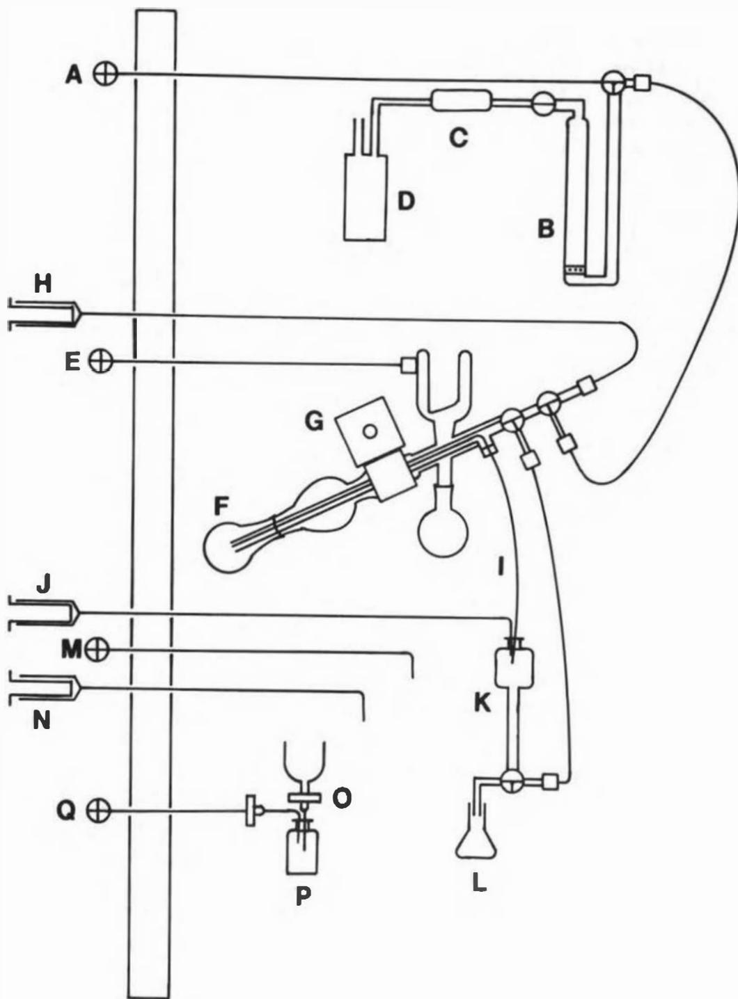
**Fig. 6** Experimental setup for 2-deoxy-2[18]fluoro-D-glucose synthesis.
