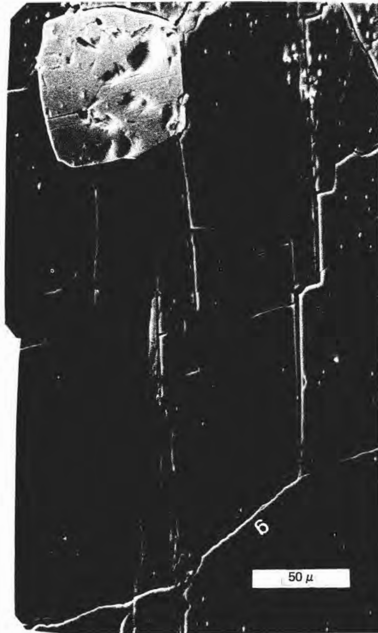
FIGURE 7a A photomicrograph of Westerly granite at a stress well below the fracture strength. 6 Note that cracks have begun to extend and that the fracture is brittle.
