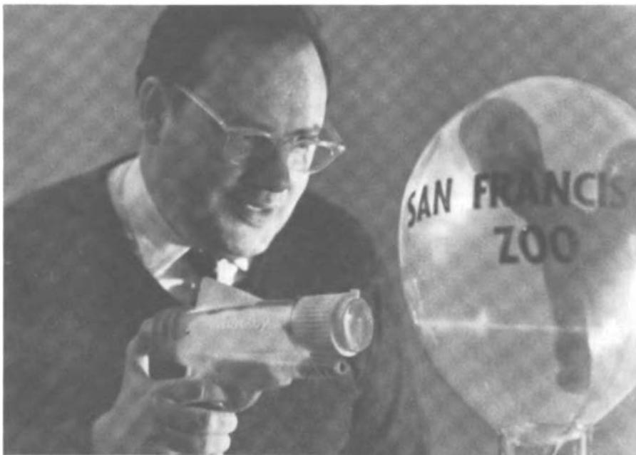
FIGURE 3 A flash of light from a ruby laser breaks the blue inner balloon without harming the clear outer balloon.
