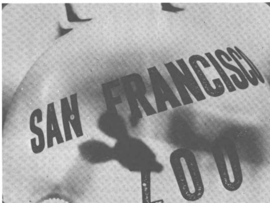
FIGURE 5 Balloon after the laser eraser has erased a spot from the letter N.
