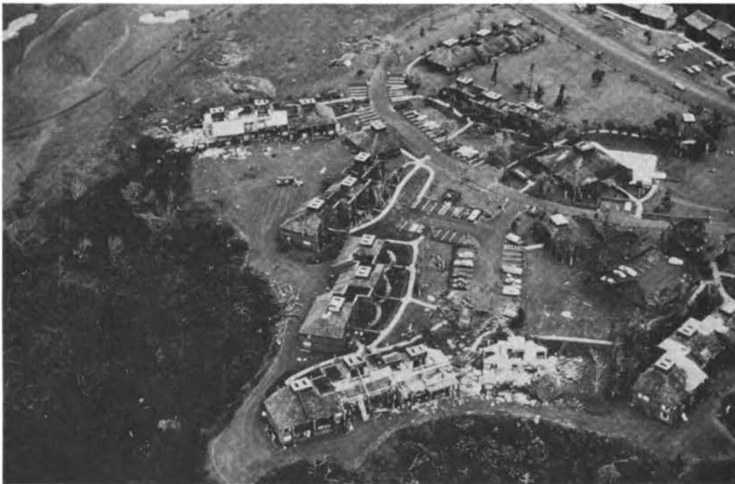
FIGURE 3.64 Damage at Pali Ke Kua, Princeville, Kauai (note damage to units sited near bluffs).
