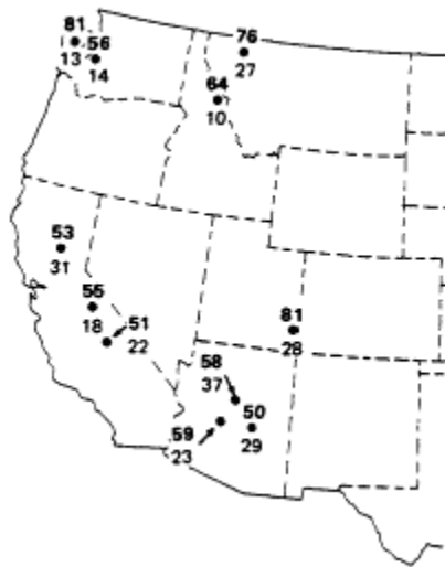
Figure 4B-5 Observed point rainfalls exceeding 50% of all-season PMP, west of continental divide for 1,000 square miles and duration between 6 and 72 hours. (Large number is the percentage of the PMP, small number is storm index.) Source: U.S. Army Corps of Engineers (1982b).
