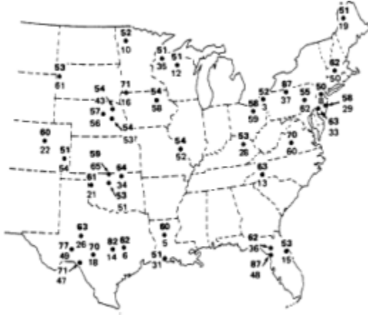
Figure 4B-2 Observed point rainfalls exceeding 50% of all-season PMP, east of 105th meridian for 200 square miles, 24 hours. (Large number is the percentage of the PMP, small number is storm index.) Source: U.S. Army Corps of Engineers (1982b).
