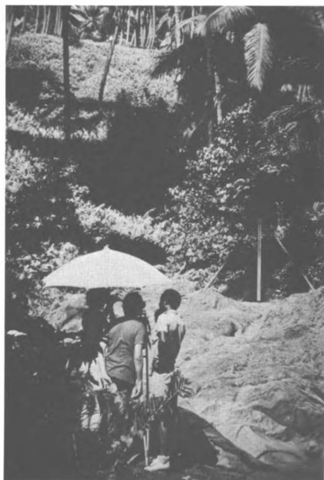
FIGURE 13.5 Dry tilt measurements being made on St. Vincent in March 1977, more than 2 yr before the 1979 eruption. Data obtained from this station helped confirm that the volcano was inflating.
