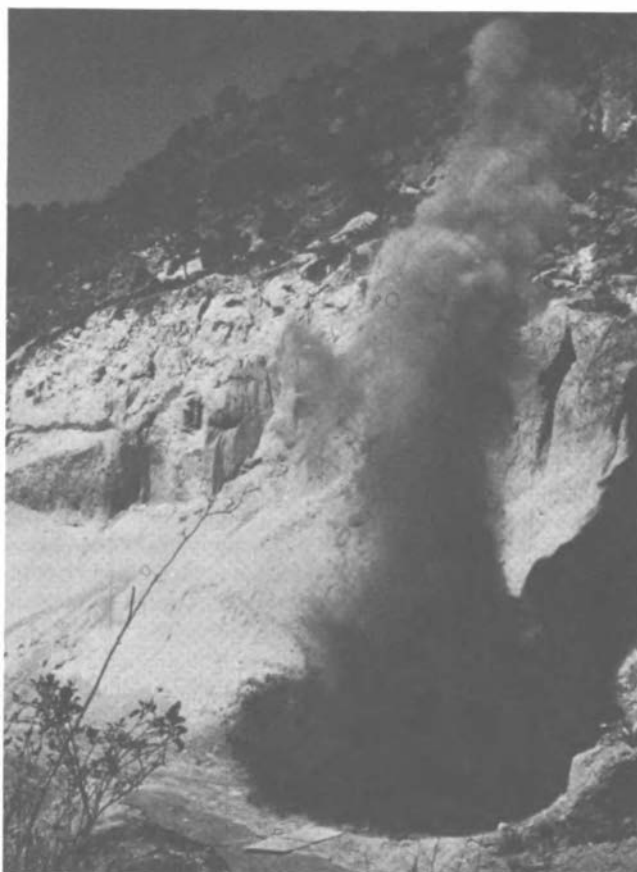
FIGURE 12.5 Experiment 1 (Table 12.1) showing vertical ejection column and horizontally expanding base surge.
