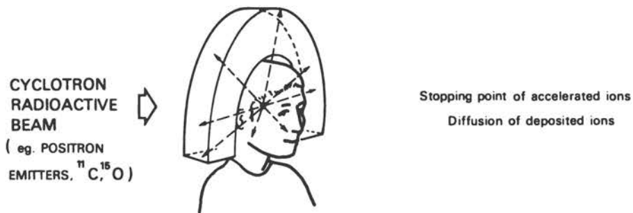
FIGURE 5 Accelerated heavy ions are used for imaging and for exploring diffusion by injection of positron emitters and simultaneous measurement of emitted annihilation photons.
