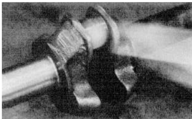
Figure 4 Co 2 laser beam being used to harden lobe surface of crankshaft. From Note 8. Reprinted with permission.
