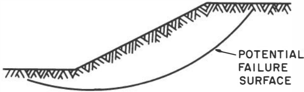
FIGURE 4-47 Hypothetical slope and potential failure surface.
