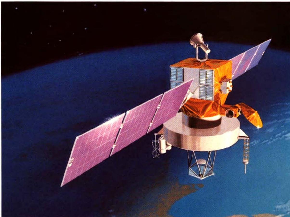
NASA SPACE RESEARCH MISSIONS PROBE GLOBAL EARTH PROCESSES. Joint U.S./France TOPEX/POSEIDON satellite will measure sea-surface topography to provide data for models of ocean circulation ( artist's conception ).
