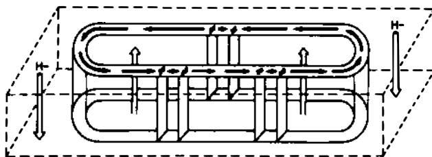
FIGURE 8.6 As described by H. Hayashi [ Hikkei Comput. 97-102 (May 30, 1983)], Nippon Electric Company's Bloch line memory is based on the magnetic structure shown here. The magnetization in the wall of a stripe domain in bubble material can rotate in either of two senses from the direction of the field inside the stripe to the direction of the field outside the stripe. If a twist is put into the wall, the sense of rotation is reversed in a small portion of the wall, and a pair of Bloch lines forms—one on either side of the twist. The existence or absence of the Bloch line pair can be interpreted as a bit of information. Theoretically, this would permit information to be stored approximately 100 times more densely than in conventional bubble memories.
