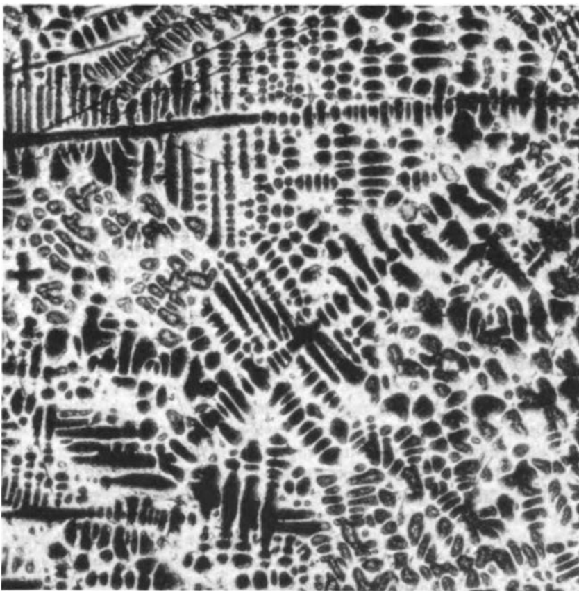
FIGURE 4.2 This complex composite structure in a metal alloy is an intimate mixture of two phases formed by dendritic growth of one of the phases during solidification.
