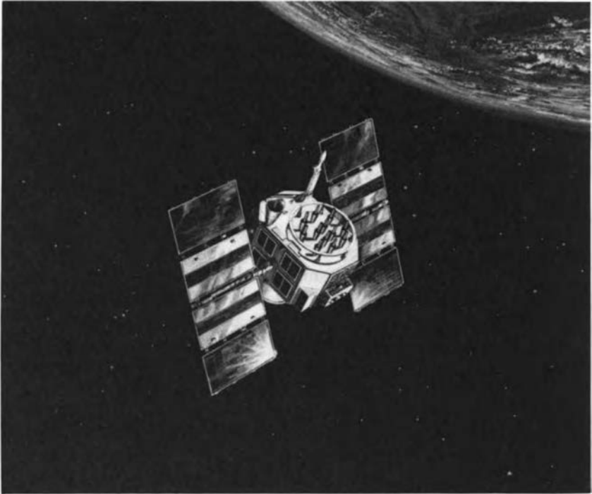
FIGURE 12.3 Global Positioning System satellites, such as the one depicted in this artist's rendition, utilize on-board rubidium atomic clocks and theory-of-relativity adjustments to provide routine navigational position fixes accurate to better than 100 m. Omission of relativistic adjustments would lead to an error accumulation of 12 km per day. (Illustration courtesy of Rockwell International.)
