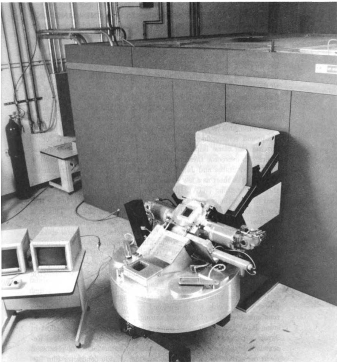
FIGURE 2. High-current ion implantation accelerator and wafer processing station used for the fabrication of buried insulating \text{SiO}_2 layers in silicon formed by \text{O}^+ implantation. Courtesy of Eaton Corporation.
