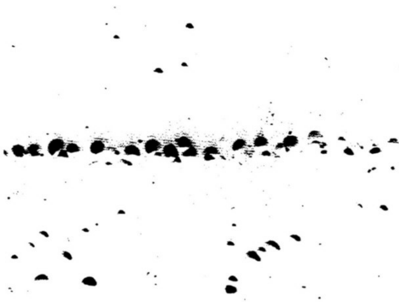
FIGURE 12 Direct evidence of dislocation arrays in crystals, derived from the etching behavior of high-purity germanium.
