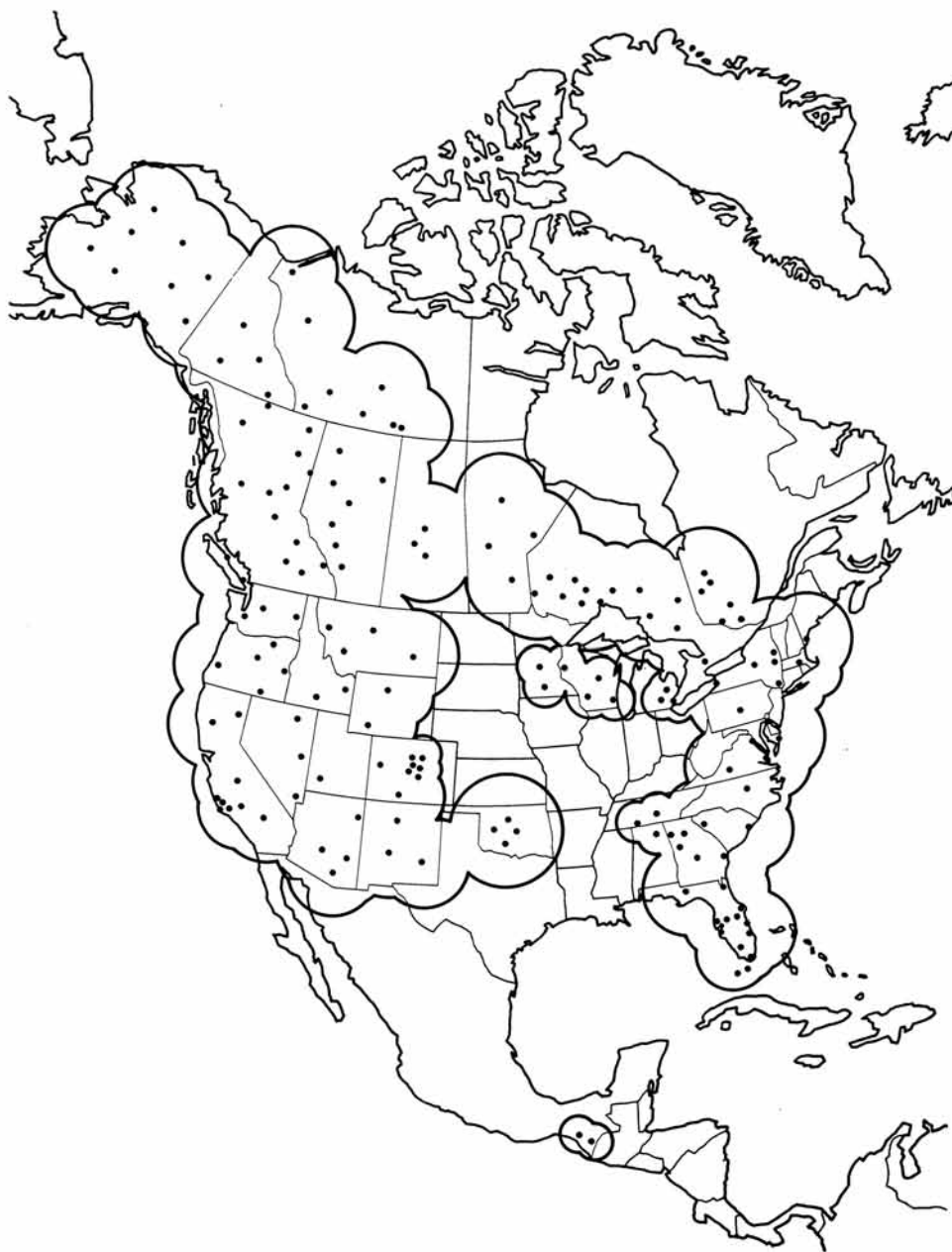
Figure 5.1 A map showing the location (dots) of lightning direction finding (DF) stations in place in summer 1984. is Connected circles around each DF indicate area of lightning coverage. The area of coverage along the East Coast is the SUNYA East Coast Network.
