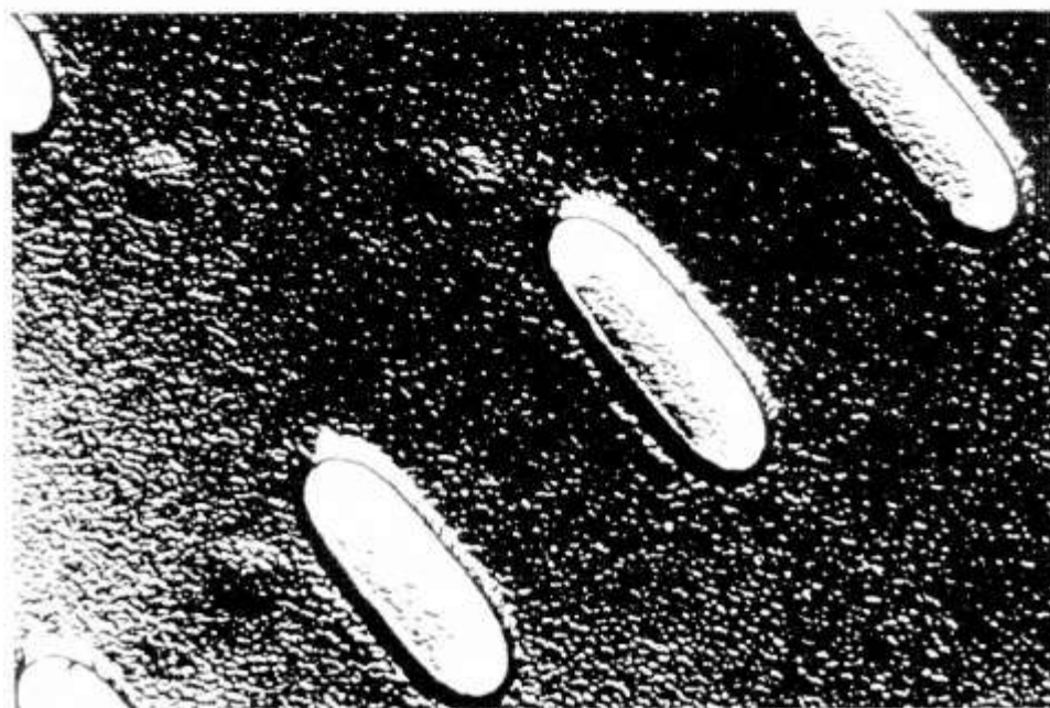
Optical disk—a recent development in data storage technology. The magnified view shows digitized data encoded on the disk.
