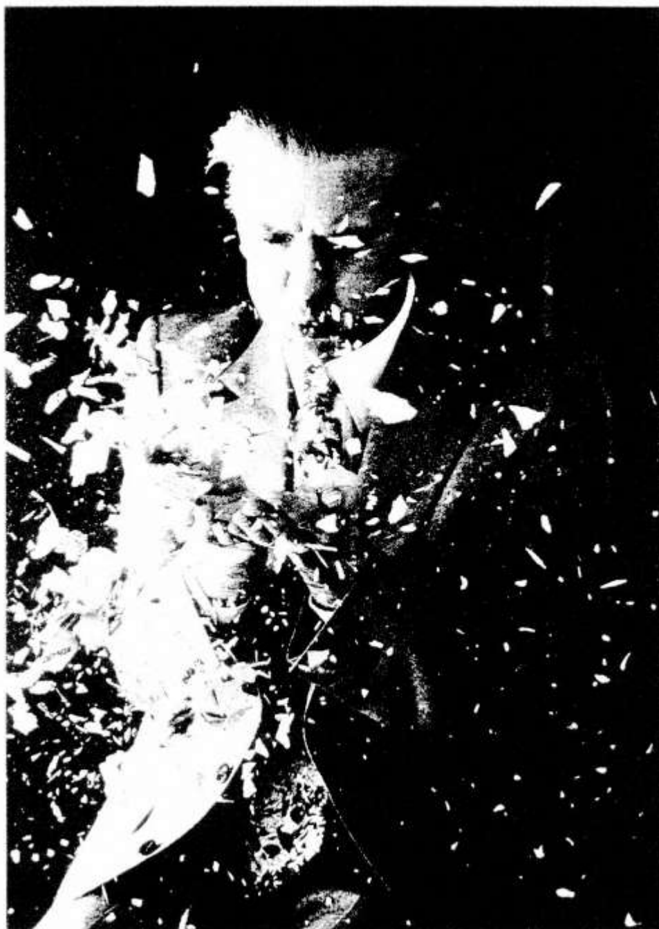
Effects of slow-working acid in book paper. Peter Waters, conservation officer at the Library of Congress, demonstrates that a hefty puff makes confetti of deteriorated pages.
