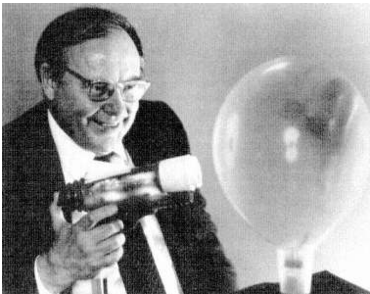
Figure 1 Arthur L. Schawlow demonstrating that a flash of red light from a small ruby laser breaks the dark-colored inner balloon without damaging the transparent outer balloon. This procedure exactly mimics the way laser light can be used to repair a detached retina inside the eyeball, make a weld inside a closed vacuum chamber, or trigger a chemical reaction inside a closed chemical cell. Photograph by Frans P. Alkemade.
