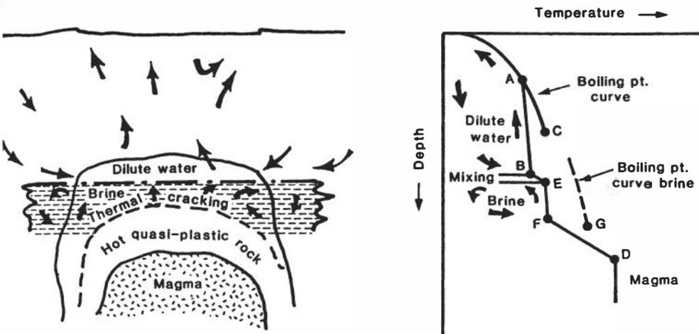
**FIGURE 8** (a) Schematic diagram showing inward crystallisation and subsequent cooling of a magmatic body beneath a silicic caldera. Brine that forms by condensation of superheated fluids, partly of meteoric origin and partly of magmatic convecting meteoric water. (b) Schematic depth-temperature profile for conditions shown in Figure 8(a).
