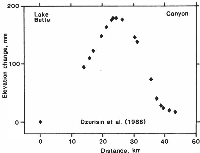
FIGURE 6 Elevation changes at Yellowstone caldera during 1976-1984 measured along the road from Canyon Junction to Lake Butte. From Dzurisin and Yamashita (1986) and Dzurisin *et al.* (1986).
