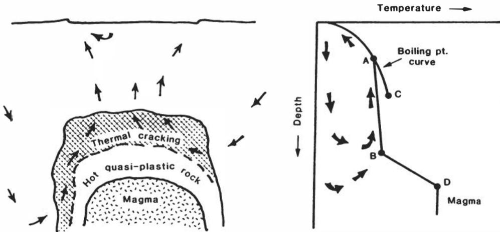
**FIGURE 7** (a) Schematic diagram showing inward crystallization and subsequent cooling of a magmatic body beneath a silicic caldera. (b) Schematic depth-temperature profile for conditions shown in Figure 7(a).
