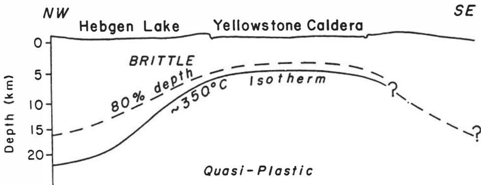
FIGURE 4 Cross section through the Yellowstone Caldera showing the contour above which 80 percent of the earthquake focal depths occur and the estimated depth to the 350°C isotherm. From R. B. Smith (University of Utah, written communication, 1985).
