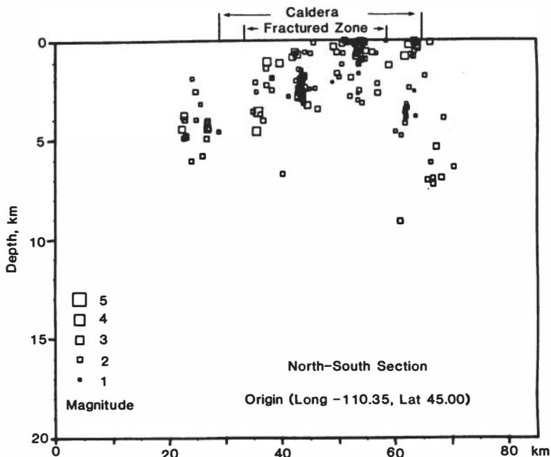
**FIGURE 3** Focal depths of earthquakes in and adjacent to the Yellowstone Caldera that can be located with above-average precision. Modified from Fournier and Pitt (1985).
