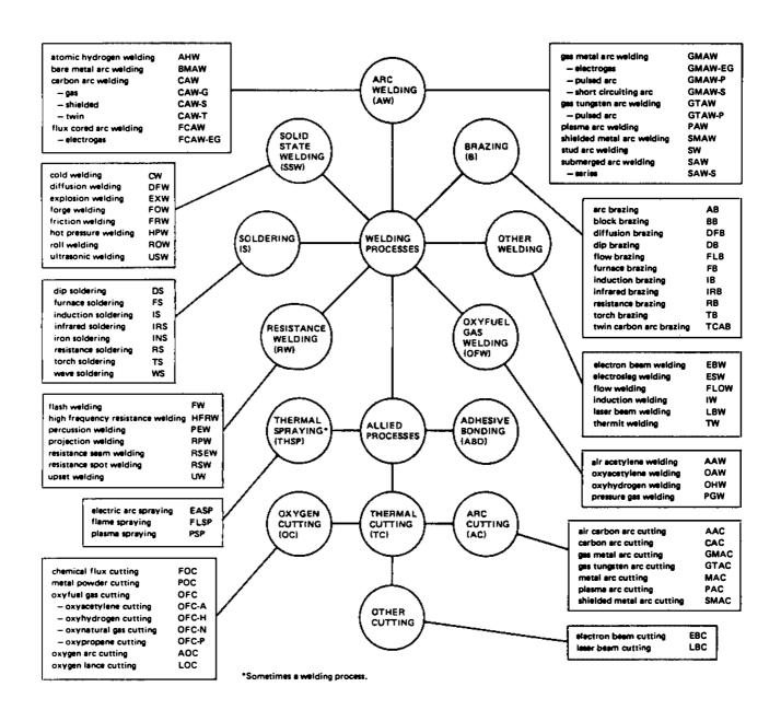
Figure 2 Welding and allied processes (American Welding Society, 1984).
