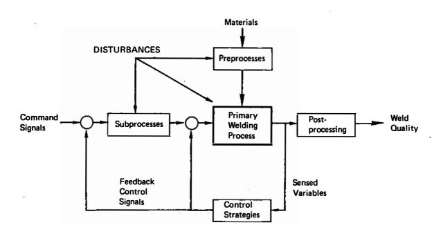
FIGURE 1 Block diagram of the welding control problem.
