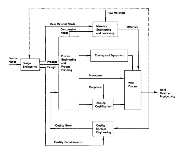
FIGURE 3 Welding manufacturing system.
