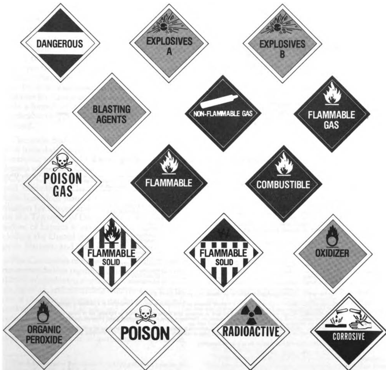
Figure 4-4.—Examples of Hazardous Materials Placards
