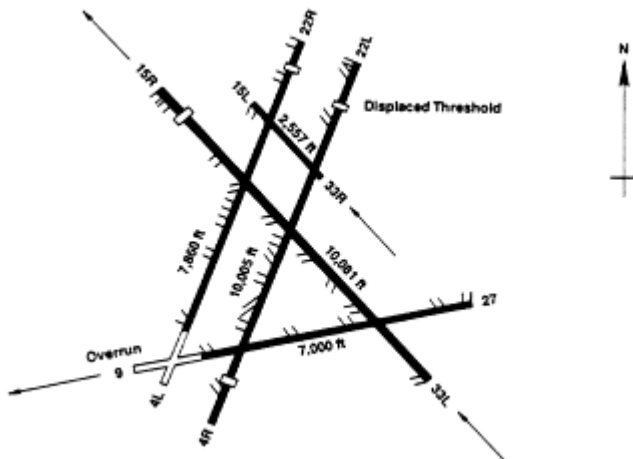
Figure 9-5 Runway operation patterns at Boston's Logan International Airport: four configurations with the west flow configuration operated 42 percent of the time.
