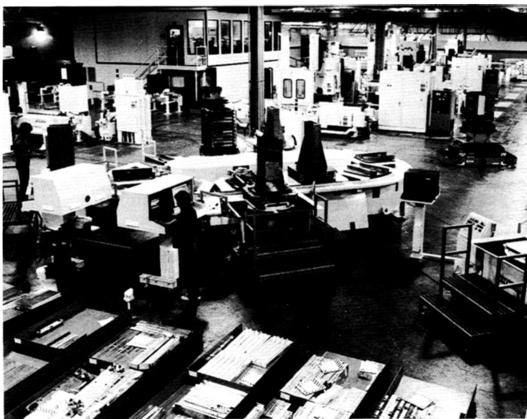
Figure 2 Flexible machining cell layout: (top) schematic, (bottom) factory-floor view.
