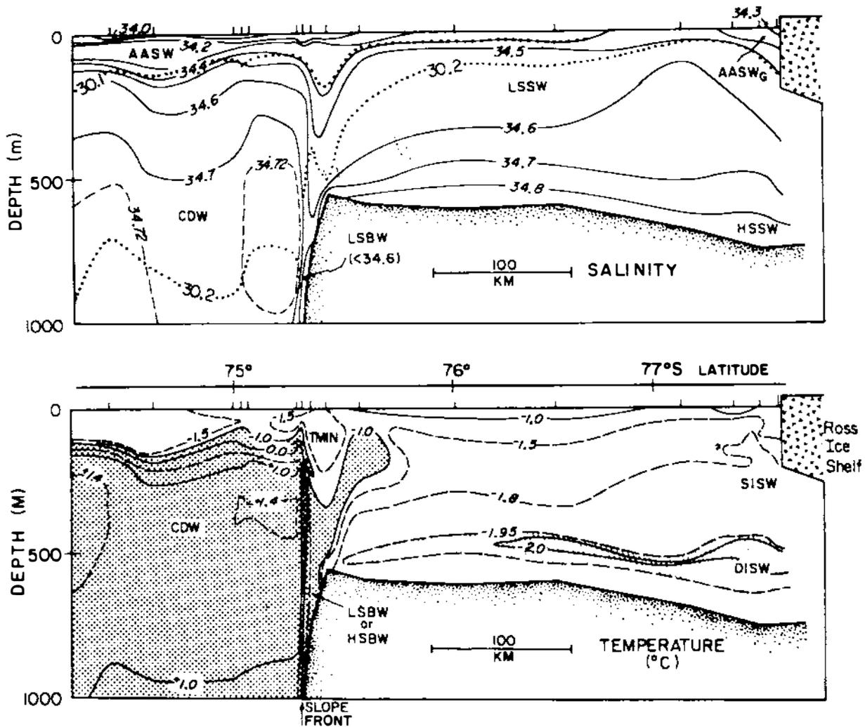
FIGURE A-8 Shelf-slope frontal zone in the Ross Sea. Salinity and temperature versus depth along transect, December 1976 STD stations. Vertical ticks indicate station locations. Dotted isopycnal surfaces in the salinity section are referenced to 500 db. At these continental shelf depths, potential temperatures would be about 0.03°C colder than the in situ temperatures shown. Source: Jacobs, et al (1985).
