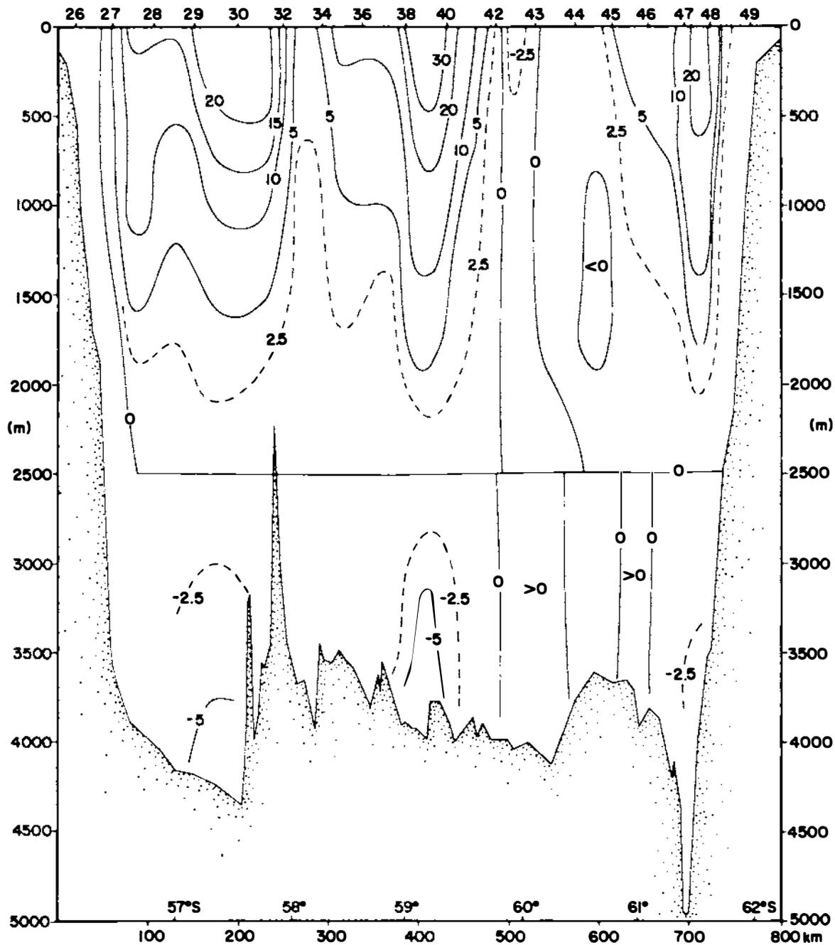
FIGURE A-6 Through-passage geostrophic speed (cm/s). Source: Nowlin, Whitworth, and Pillsbury (1977).
