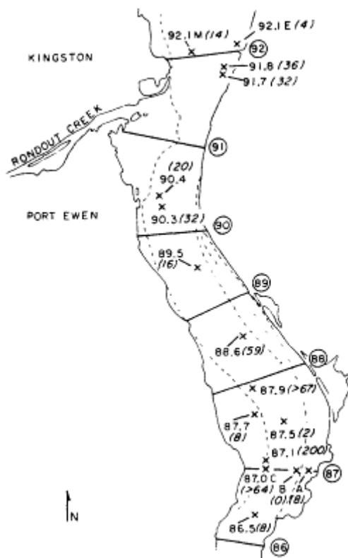
Figure 6 A map of the Hudson River from mp 86 to 93. Sediment core locations are marked with x's and labelled by mile point. Numbers in parentheses indicate the depth of penetration of Cs-137 in centimeters.
