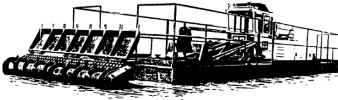
Figure 3 The Mud Cat—notice that the cover is lifted to show two augers.
