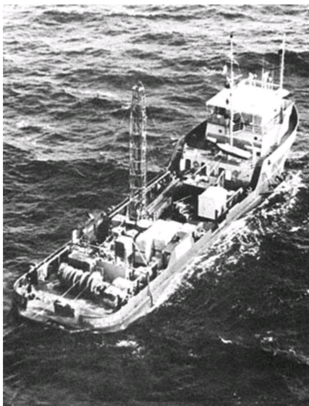
Figure 4-10 Oil field supply vessel outfitted with a portable drilling rig. Source: McClelland and Ehlers, 1986.
