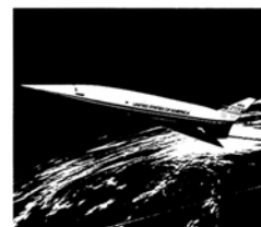
The National Aero-Space Plane flies far above the earth in an artist's drawing. New advanced composite materials are being developed for its skin, engines, and other components that will allow the space plane to climb into orbit or cruise in the atmosphere at more than six times the speed of sound.
