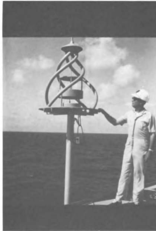
FIGURE 10 Part of the satellite positioning system on the Glomar Challenger .
