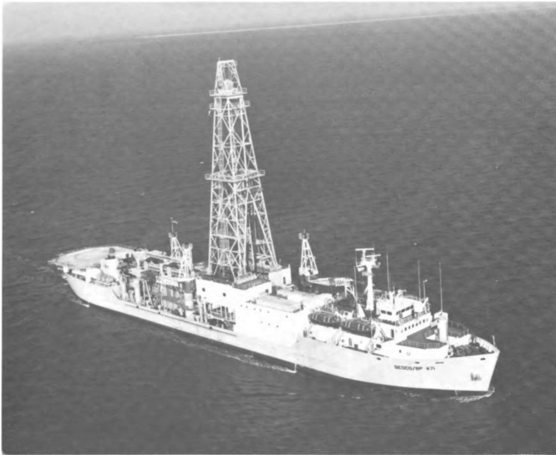
FIGURE 53 JOIDES Resolution (SEDCO/BP 471), drill ship for the Ocean Drilling Program (ODP). Note the large laboratory stack (with portholes) just forward of the derrick. The ship is 470 feet long, 70 feet wide, and the derrick rises 200 feet above the waterline. It is operated by Texas A&M University, science operator for the ODP.
