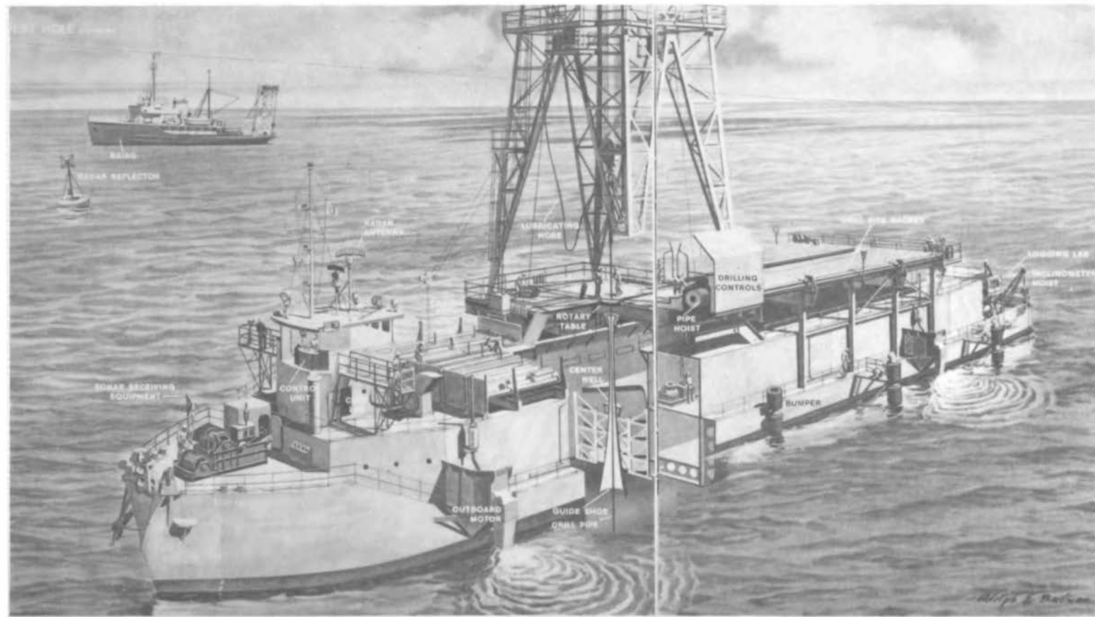
FIGURE 4 Sketch of CUSS 1 , illustrating parts of the dynamic positioning system, guide shoe, and drilling system. Diagram by Adolph E. Brotman in The Mohole: preliminary success in drilling through the earth's crust : LIFE magazine, April 7, 1961, pp. 37-40.
