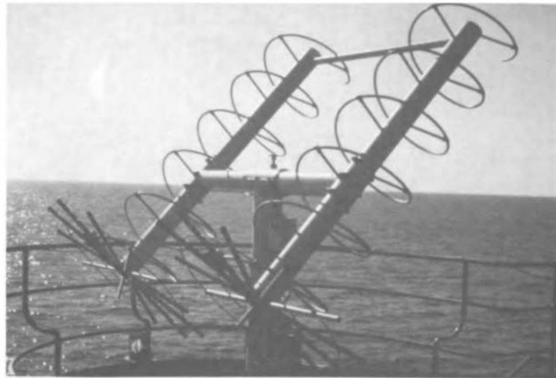
FIGURE 11 Receiving apparatus for the satellite communications system.
