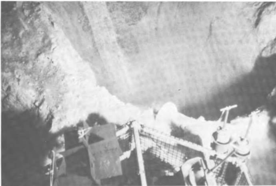
FIGURE 14 Hole in the seafloor created by drilling. Photo taken by the ALVIN.
