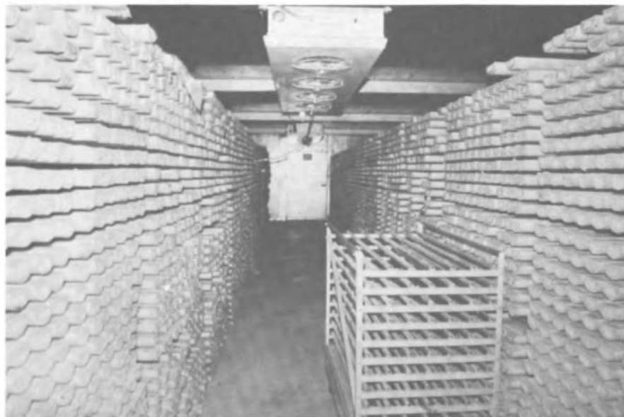
FIGURE 18 Core storage facility. The cores are placed in plastic containers and the temperature is maintained at just above freezing.
