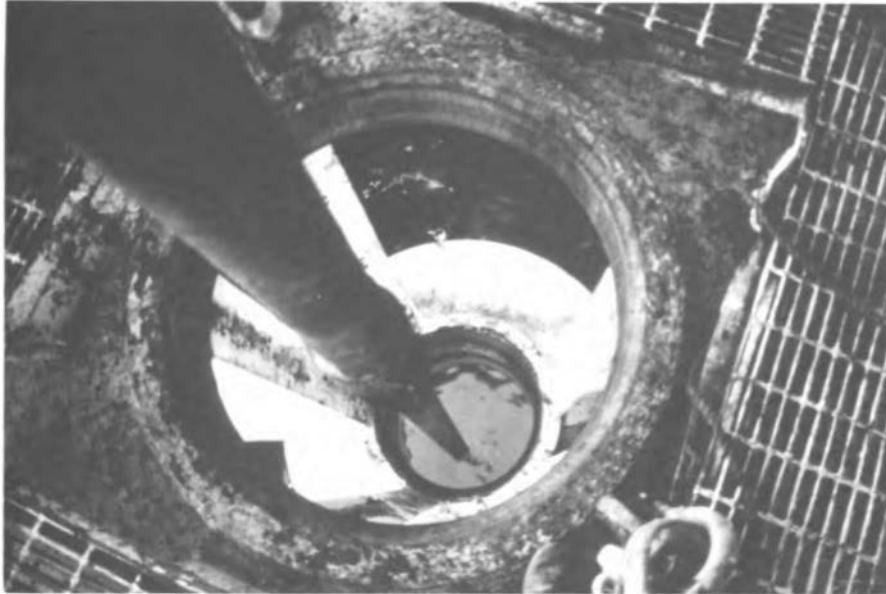
FIGURE 13 The drill string passing through the moon pool.
