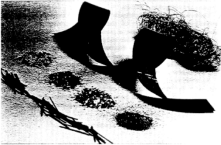
Figure 2.7 Metallic glass product forms. (Reprinted, by permission, from Battelle. Copyright (c) 1989 by Battelle Memorial Institute.)
