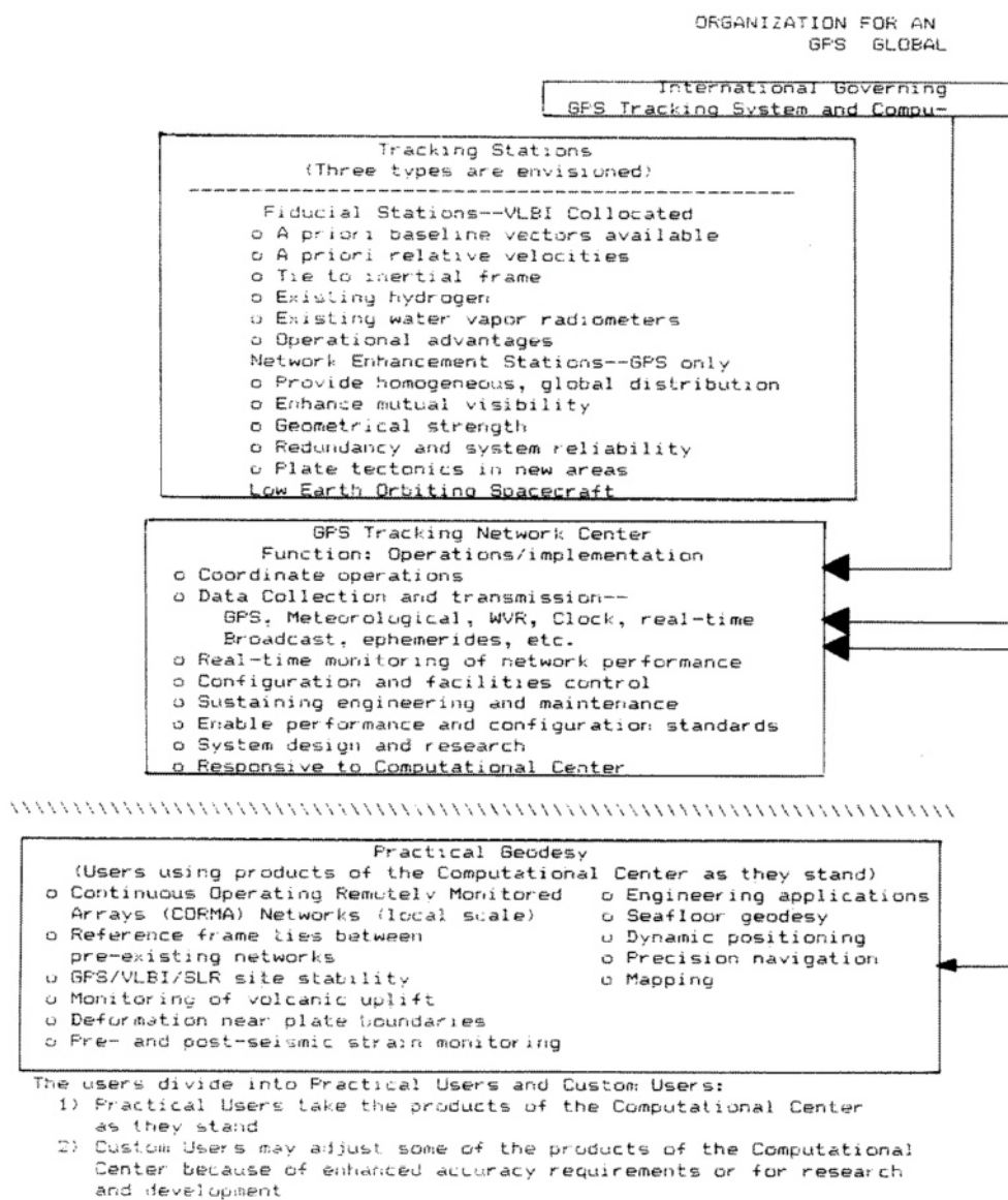
Figure 12. Organization Diagram for an Internationally Operated Civilian GPS Global Tracking System for High Accuracy Applications
