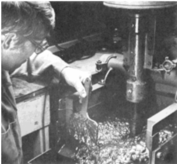
Laboratory flotation test to produce a sulfide mineral concentrate containing cobalt, 1988. (Courtesy Bureau of Mines, Albany Research Center.)
