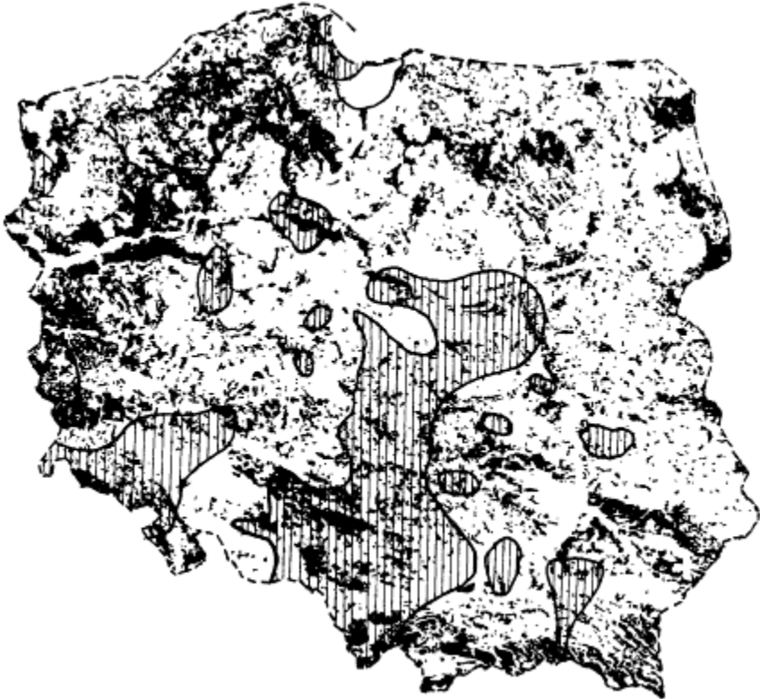
Figure 11 Distribution of coniferous and mixed forests and air pollution in Poland. The map was elaborated at the Institute of Geodesy and Cartography in Warsaw under the supervision of Andrzej Ciolkosz on the basis of Landsat MSS and Salut-6 images acquired in 1978. The isolines delimit the area with \text{SO}_2 mean annual concentration equal/higher than 50 micrograms per \text{m}^3 ; dark areas show regions above 150 micrograms. Data on pollution from the map predicting air pollution in Poland in 1990 by J. Juda et al., 1982 (manuscript).
