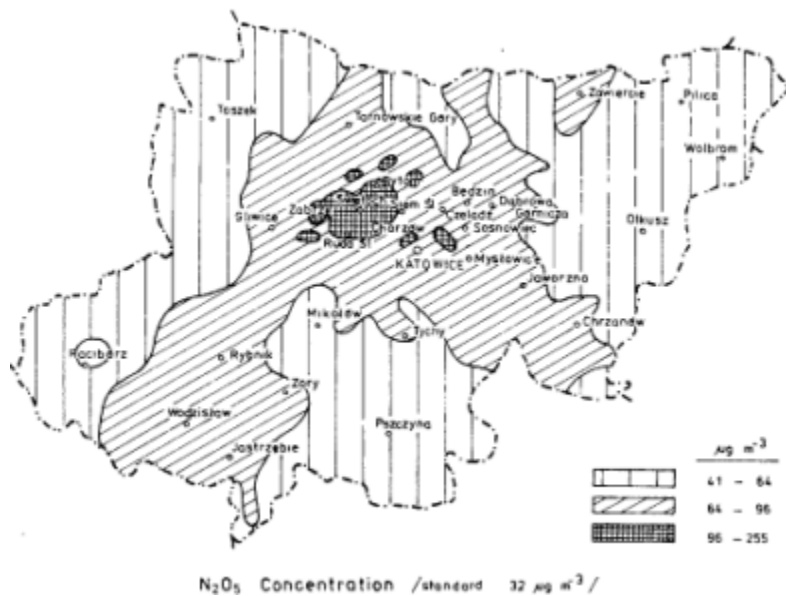
Figure 4 Concentration of nitrogen oxides in the Katowice district with yearly mean values (in \mu\text{g m}^{-3} ). The permissible concentration (national standard) is 32 \mu\text{g m}^{-3} (District Office for Public Health and Epidemiology, Katowice).
