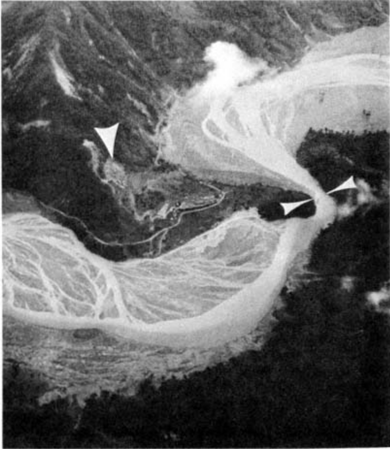
FIGURE 5.16B floodplain. Bedrock constriction of the Coca River (indicated by two arrows at the right) probably caused short-lived "hydraulic" damming of the river that contributed to upstream flooding and sedimentation. Note landslide (single arrow near center of photo) that badly damaged the Salado pumping plant of the Trans-Ecuadorian oil pipeline.
