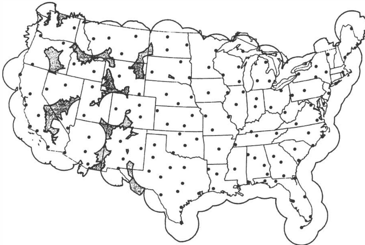
**FIGURE 1** Locations and total coverage (at 3,000 m elevation) of the national NEXRAD network. Shaded areas represent gaps, mostly in mountainous areas, in NEXRAD coverage. (Reprinted with permission of the National Weather Service.)
