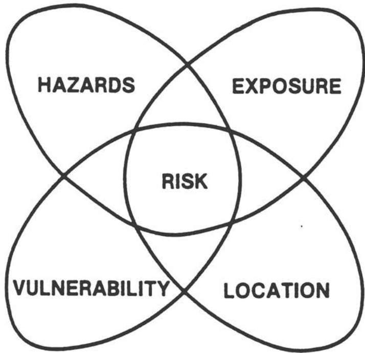
Figure 3. The risk at a location is a function of the vulnerability of buildings and lifeline systems exposed to the ground shaking and ground failure generated in an earthquake.
