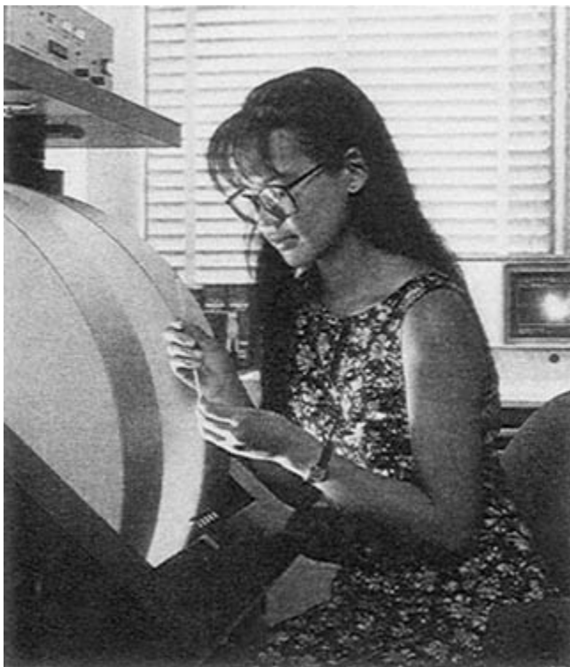
Precise measurements of absorbed radiation dose for industrial and medical applications can be made at the NIST Electron Paramagnetic Resonance Facility. Here, physical science trainee Francoise Le inserts a bone fragment into the sample chamber. (Photo: H. Mark Helfer, National Institute of Standards and Technology)
