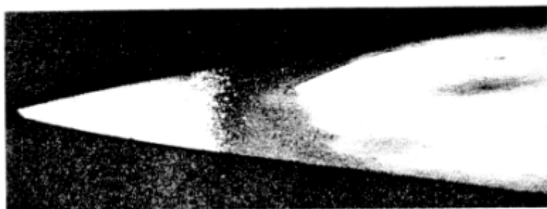
Figure 3-7 Cross-section of a Japanese sword blade (18th century). The white area near the edge is martensite. This merges gradually into dark-etching pearlite and a soft iron core.
