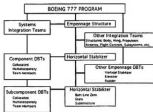
Figure 2-3 An example of a typical structures DBT hierarchy: Boeing 777 Horizontal Stabilizer DBTs. Source: Boeing Commercial Airplane Group.
