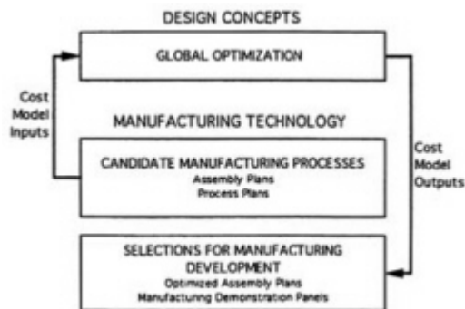
Figure 2-5 The interactions of a typical DBT during initial concept development. Source: Boeing Commercial Airplane Group.
