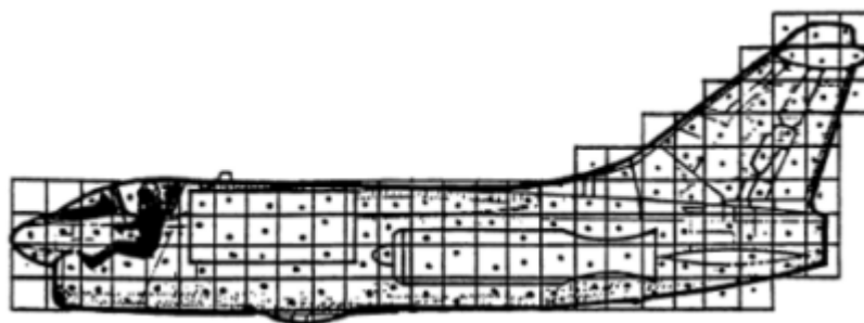
Figure 1-2 Example of a grid and random shotlines from FASTGEN for COVART (Ball, 1985). Copyright © AIAA 1985—Used with permission.
