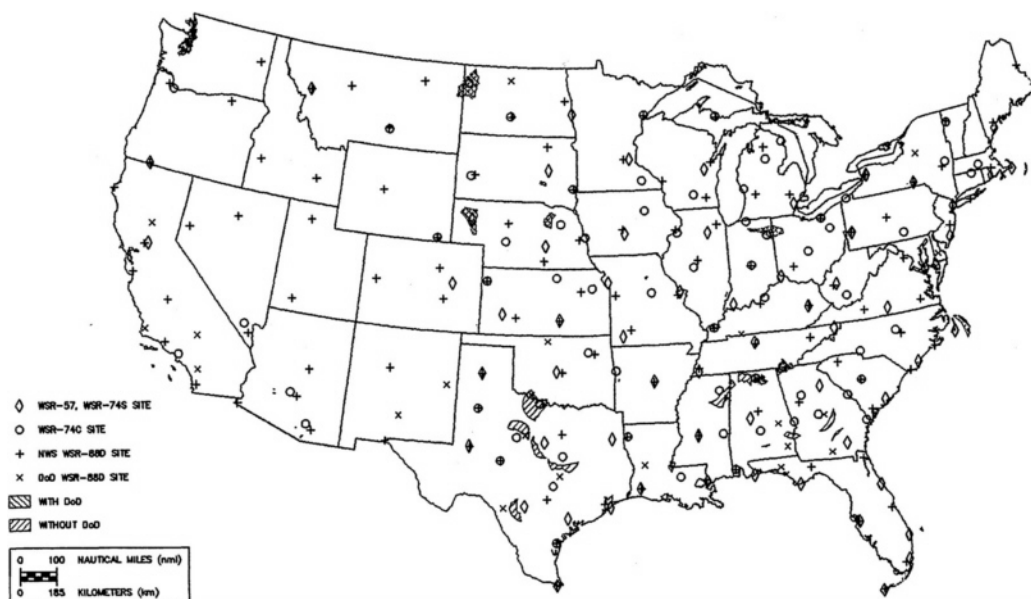
Figure 2-3b Areas with potentially degraded detection coverage for supercells by NEXRAD with DoD (red) and without DoD (blue) NEXRADs compared with the pre-NEXRAD radars. The pre-NEXRAD radars relied on the “hook echo” for supercell detection, while the NEXRAD detects mesocyclone circulation. Courtesy of SRI International.
