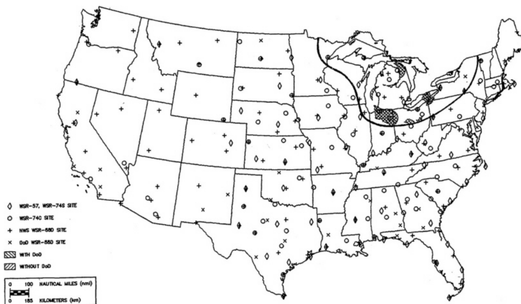
Figure 2-6b Areas with potentially degraded detection coverage for lake effect snow by NEXRAD with DoD (red) and without DoD (blue) NEXRADs compared with the pre-NEXRAD radars. The solid black line marks the boundaries on each map for the areas that have a significant risk of lake-effect snow. Courtesy of SRI International.
