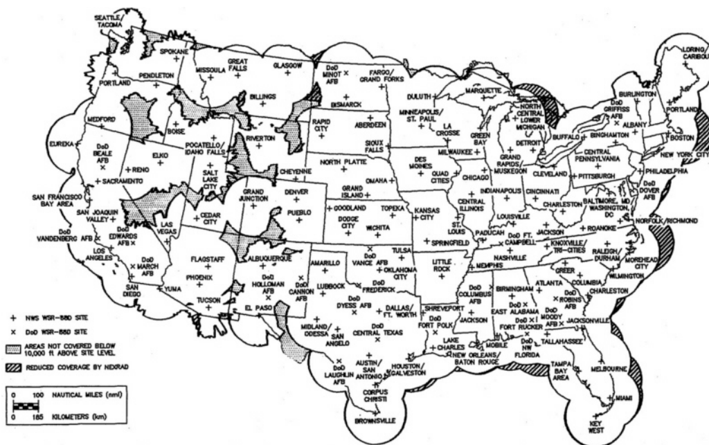
Figure 2-1b Composite NEXRAD coverage at 10,000 ft above site level for the contiguous United States and the locations of NWS and DoD sites. This figure also shows those areas (striped blue) where there will be reduced coverage at 10,000 ft by the NEXRAD network compared with that which existed with the pre-NEXRAD network, as specified in P.L. 102-567, Sec. 702(4). Courtesy of SRI International.
