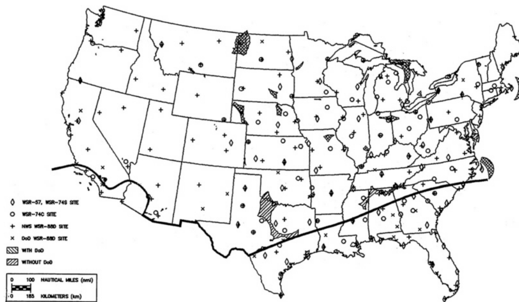
Figure 2-7b Areas with potentially degraded detection coverage for stratiform snow by NEXRAD with DoD (red) and without DoD (blue) NEXRADs compared with the pre-NEXRAD radars. The solid black line marks the boundaries on each map for the areas with a significant risk of stratiform snow occurring. Courtesy of SRI International.
