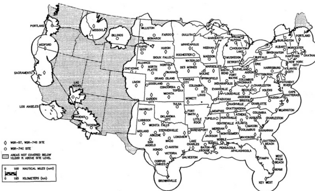
Figure 2-1a Composite pre-NEXRAD coverage at 10,000 ft above site level for the contiguous United States and the locations of the radars by type. Courtesy of SRI International.
