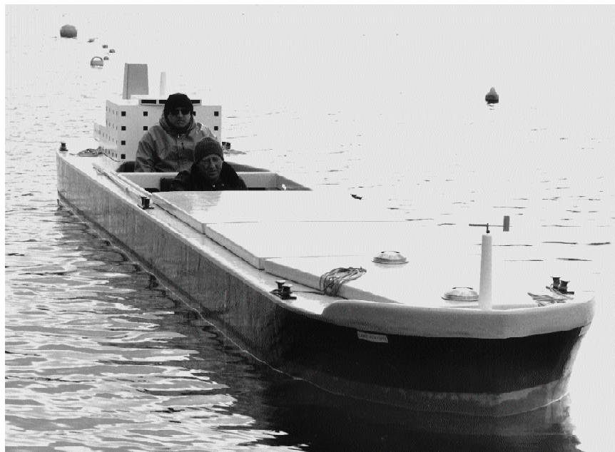
FIGURE 2-6 An example of a manned-model simulator. (The Southampton Institute, Warsash Maritime Centre, United Kingdom)
