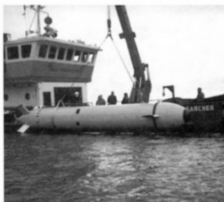
FIGURE 1-8 Photo of Theseus (International Submarine Engineering, Ltd.). Theseus is a multipurpose autonomous underwater vehicle developed by International Submarine Engineering, Ltd. for the Canadian Defence Research Establishment Pacific. The vehicle is undergoing test trials. Operations to 1,000-meter depth extending up to 350 kilometers have been demonstrated. Source: International Submarine Engineering, Ltd.
