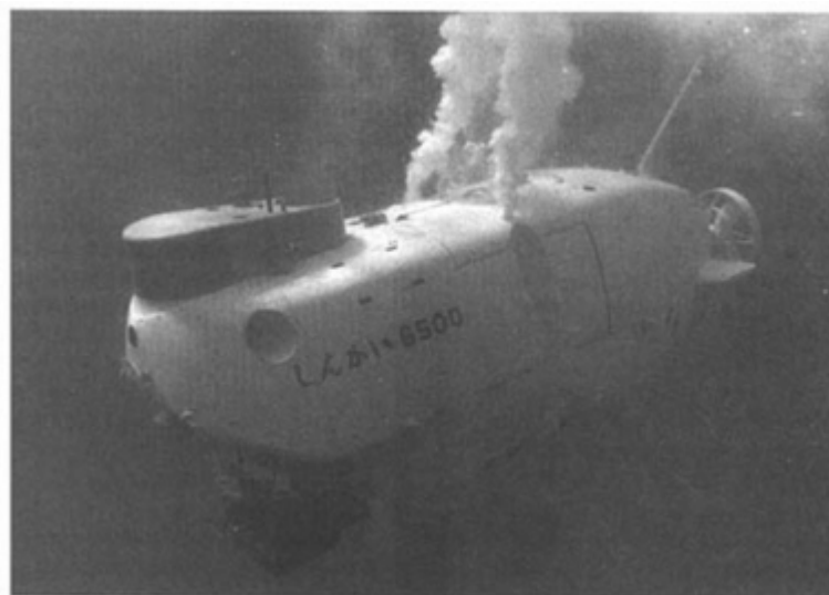
FIGURE 1-11 Photo of Shinkai (Mitsubishi Heavy Industries/Japan Marine Science and Technology Center). Shinkai 6500 was built by Mitsubishi Heavy Industries, launched in 1989, and is operated by Japan Marine Science and Technology Center. Shinkai 6500 carries a crew of three and is capable of diving to 6,500 meters, making it the deepest diving DSV in the world. Source: Japan Marine Science and Technology Center.
