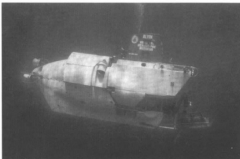
FIGURE 1-1 Photo of Alvin (Woods Hole Oceanographic Institution/Navy). The U.S. Navy-owned Alvin has been operated by the Woods Hole Oceanographic Institution since 1964. Its depth capability is 4,500 meters. It carries a crew of three and has made over 3,000 scientific dives. Source: Woods Hole Oceanographic Institution.
