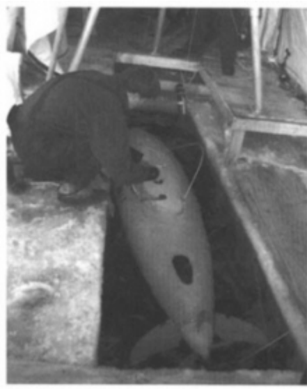
FIGURE 1-9 Photo of Odyssey I (Massachusetts Institute of Technology). Odyssey I , which was launched in 1992, is the first in a series of small AUVs designed and operated by the Sea Grant Undersea Vehicles Laboratory to map under ice fields and respond to volcanic events near ocean ridges. Operational depth is 6,000 meters, and displacement is 195 kilograms. Source: Massachusetts Institute of Technology Sea Grant.
