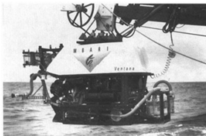
FIGURE 1-5 Photo of Ventana (Monterey Bay Aquarium Research Institute). This vehicle conducts a variety of oceanographic research tasks in biology, geology, and chemistry, to depths of 1,850 meters. Operational since 1988, it has made over 900 research dives and has logged more than 5,000 hours under water. Source: Bruce H. Robinson, Monterey Bay Aquarium Research Institute.
