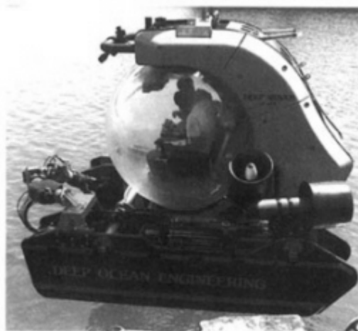
FIGURE 1-2 Photo of Deep Rover (Deep Ocean Engineering, Inc.). Two Deep Rover 1002s were built by Deep Ocean Engineering, San Leandro, California, in 1994 and delivered to a French television production company. These are two-person DSVs, designed to operate to 1,000 meters. Source: Deep Ocean Engineering, Inc. *Registered trademark of Deep Ocean Engineering, Inc.
