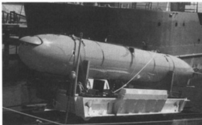
FIGURE 1-6 Photo of UUV II (Charles Stark Draper Laboratory for DARPA). The DARPA-U.S. Navy testbed unmanned, undersea vehicle was designed and built by the Charles Stark Draper Laboratory. Two vehicles have been built and are intended to validate enabling technologies for the Navy's tactical acoustical system and the autonomous mine-hunting and mapping mission. Source: Charles Stark Draper Laboratory, Cambridge, Massachusetts.
