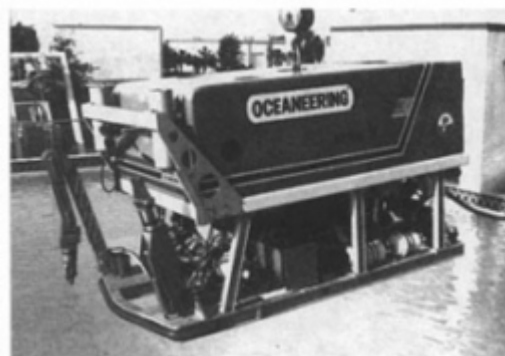
FIGURE 1-4 Photo of Triton 19 (Perry Tritech). The Perry Tritech Triton 19 is designed for operations to 1,000 meters deep and weighs 2,450 kilograms in air. Triton 19 , which has a 227-kilogram payload capability, began operations in 1994 in support of the Shell Auger Tension Leg Platform in the Gulf of Mexico. Source: Perry Tritech, Inc.
