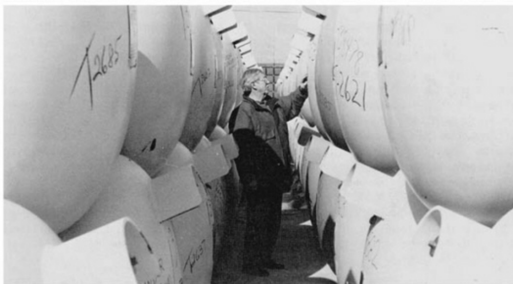
FIGURE 7-2 Cylinders stored at Portsmouth. (Cylinders are stacked to facilitate visual and ultrasound inspection.)
