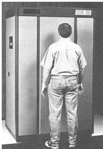
FIGURE 3-4 Person being scanned (front image) using the SECURE 1000 active x-ray imaging system produced by Nicolet Imaging Systems. Reproduced courtesy of Nicolet Imaging Systems (1995).
