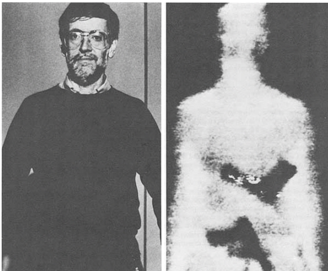
FIGURE 3-3a Visual image of a person being scanned by the Contraband Detection System produced by Millitech.
