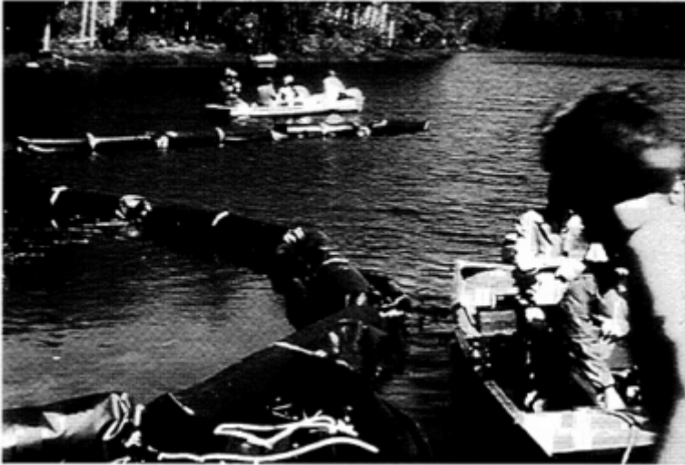
Vinyl curtain being placed in a lake for an experiment on acidification. The curtain divides the lake into two basins. One will be treated to lower the pH, and the other will be used as an experimental control. SOURCE: Dave Cornelius, University of Wisconsin, Center for Limnology.
