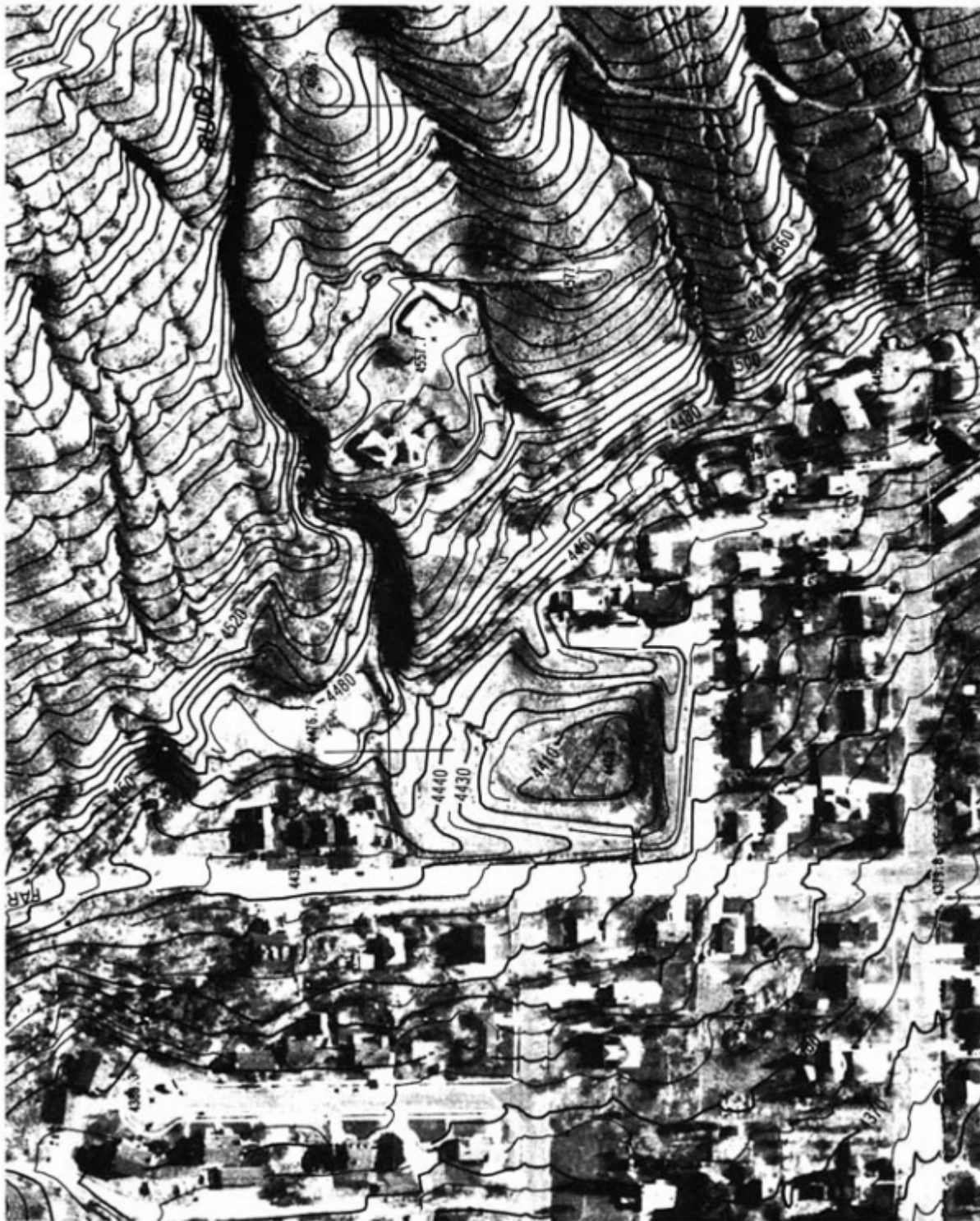
FIGURE 4-12 Topographic map on orthophoto base of Rudd Creek Canyon. The debris basin shown near the center of the map was built where homes were destroyed during the 1983 debris flow. Courtesy of Aero-Graphics, Inc.
