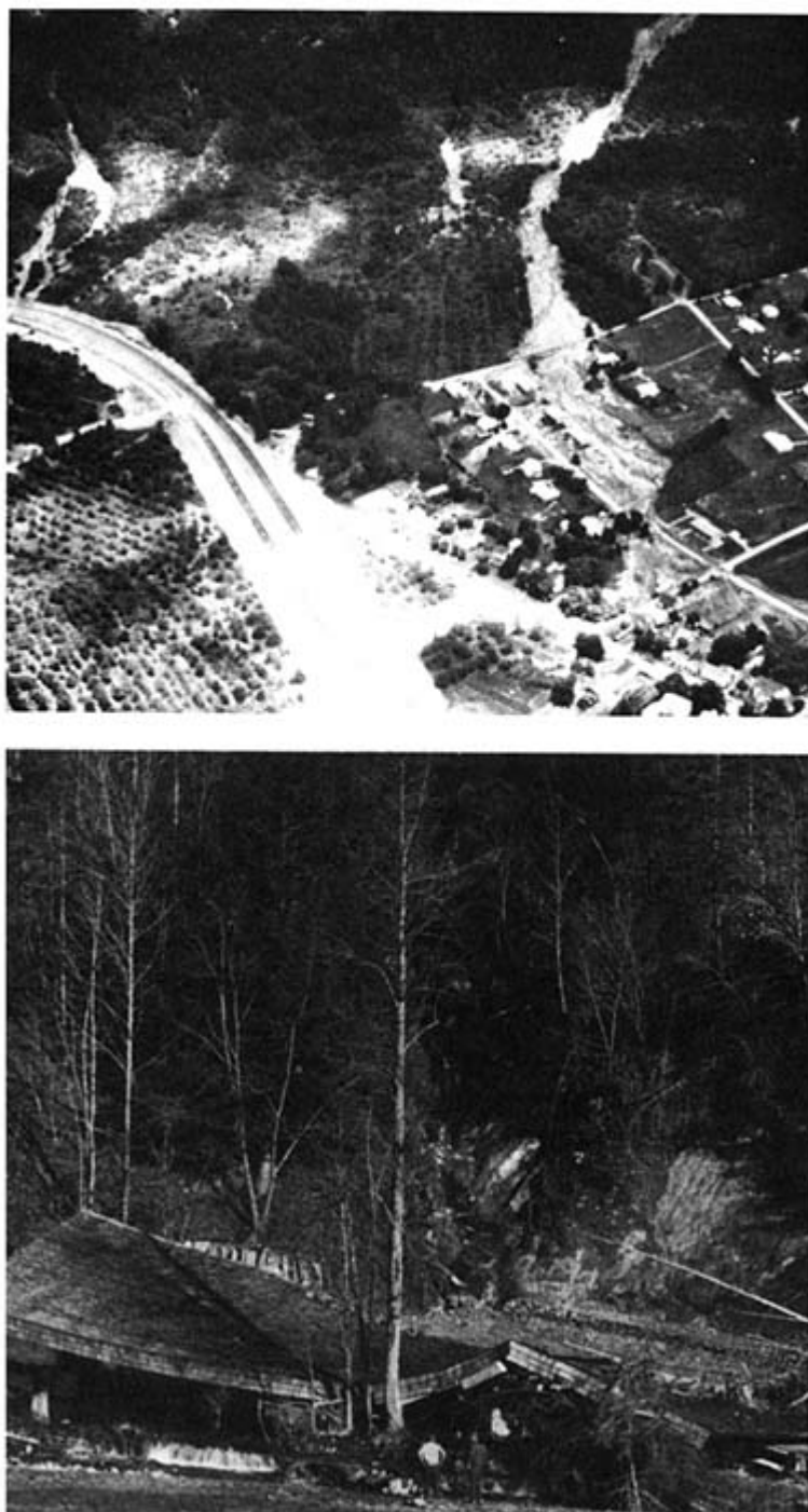
FIGURE 4-15 (Top) The town of Lovingsston, Virginia, is developed on a debris fan at the base of a debris avalanche that failed during Hurricane Camille on August 20, 1969. (Bottom) This clubhouse located on a debris fan was destroyed during a Blue Ridge, Tennessee, storm in 1973. At the time of the storm, the clubhouse was unoccupied. Upstream failure in the colluvial hollow resulted from failure of an access road fill built on the hollow. SOURCES: (Top) Williams and Guy (1973); photograph by Ed Rosenberry. (Bottom) Reprinted with permission from Clark (1987).
