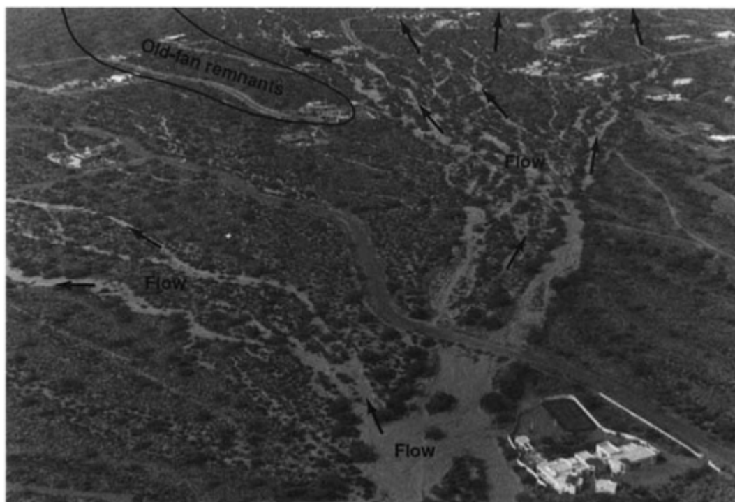
FIGURE 2-4 Oblique aerial photograph of an alluvial fan of the western slopes of the McDowell Mountains in central Arizona showing recent separation and braiding of channels downfan. The topographic apex is at the lower edge of the scene. Floodflow can inundate much of the area in the scene except for a few ridges of old fan remnants. Courtesy of H. W. Hjalmarsen.
