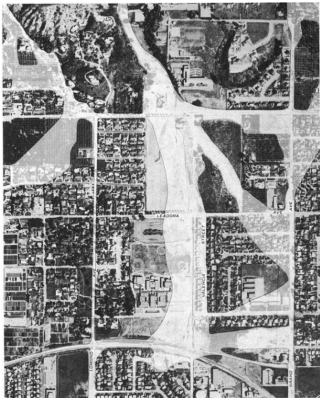
FIGURE 2-7 In urbanized settings, such as on the Glendora fan in California, streets can influence the path of floods. This area flooded in January 1969. SOURCE: Giessner and Price (1971).
